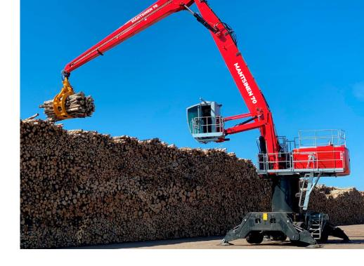
For more than two decades, Mantsinen has paved the way in energy-saving innovations and sustainable solutions. The machine has an energy-efficient, function-specific "power on demand" load-sensing LUDV hydraulic system. Additionally, the closed-loop swing hydraulics return kinetic energy back into the system during swing deceleration. The thermostat-controlled hydraulic fans run with optimum speed, thus saving power and keeping noise levels down.
