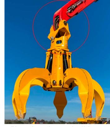
Utilizing Mantsinen attachments together with the Mantsinen material handling machines provides a clean package minimizing the chances of hydraulic hoses and electrical wires getting snagged during the operation, as all of the connections are routed through the open end of the stick and through the openings on the link and rotator packages.
